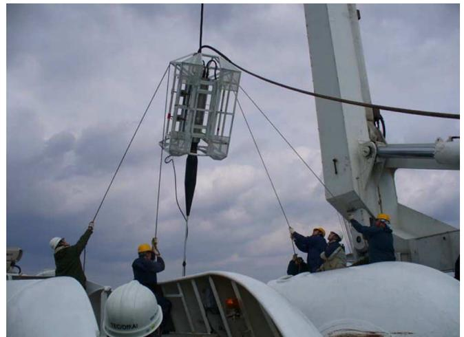
Fig. 15. Junction unit just before being paid out.
