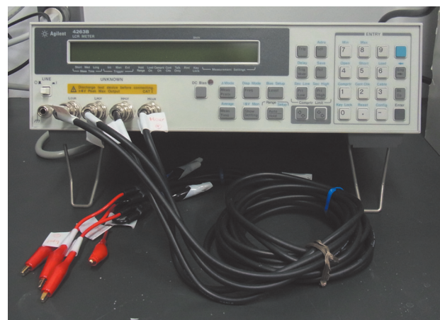
Fig. 1. Resistivity measurement system (Agilent 4263B)
