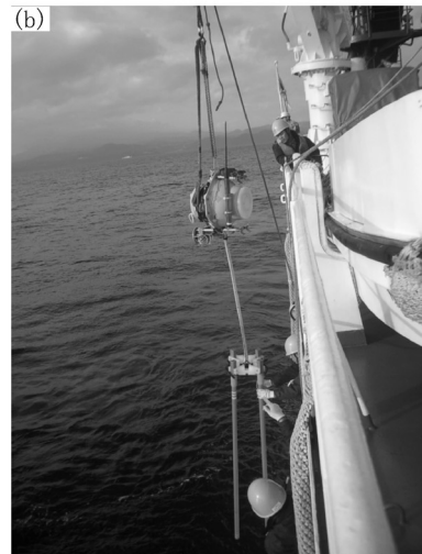
Fig.5 Photos of onboard operation (a) Deployment of OBEM system (b) Recovery Operation of OBEM system.
