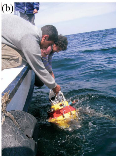
Fig. 3 (a) Deployment of the developed OBEM instrument. (b) Photograph of the recovery operation using a small fishing boat.
