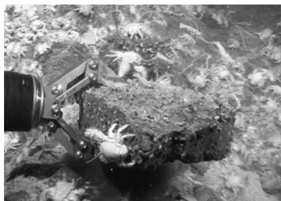
Fig. 1. Photograph at sampling of an exposed rock on the seafloor with the ROV's manipulator.
