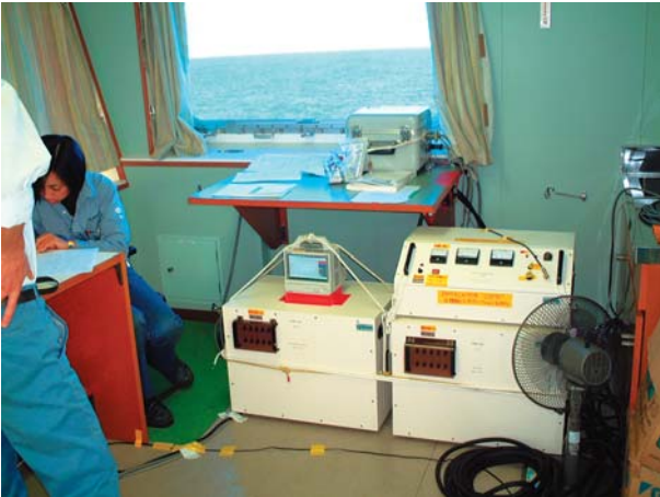
Fig.12 On board transmitter and power units for the electric current used for the MMR experiment.
