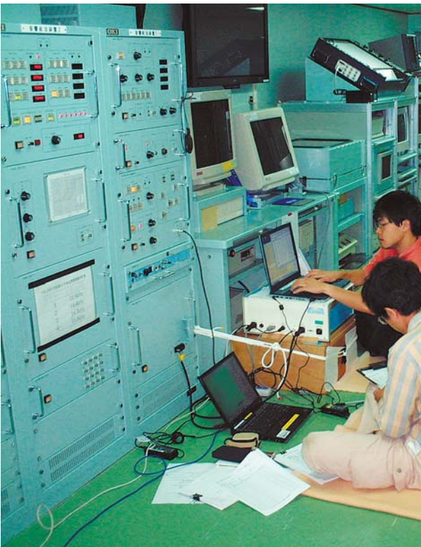
Fig.14 Acoustic unit on board (right) and Kairei's SSBL system (left) for positioning the bottom electrode.
