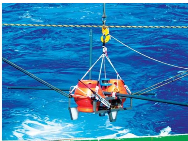
Fig.10 The outside appearance of Kobe-type OBEM with pipes for the electrodes used for the MMR experiment.
