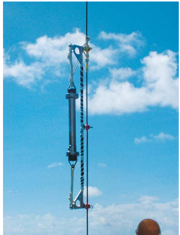
Fig.15 Acoustic unit (so called, "fish") fixed at 100 m above the bottom electrode for positioning the bottom electrode.
