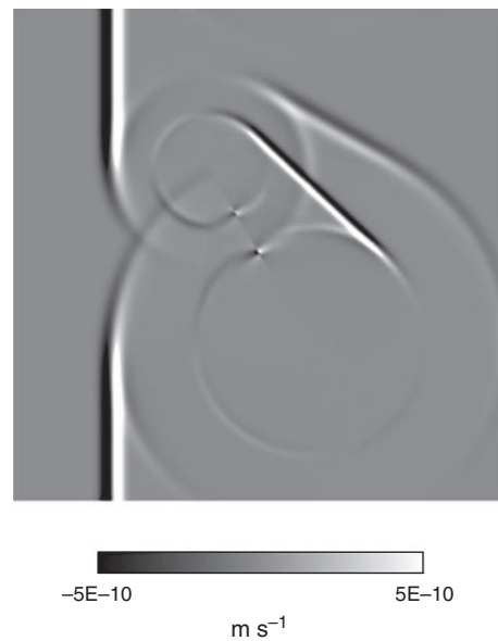
Fig. 4. A snapshot of the horizontal displacement velocity calculated by HPM.
